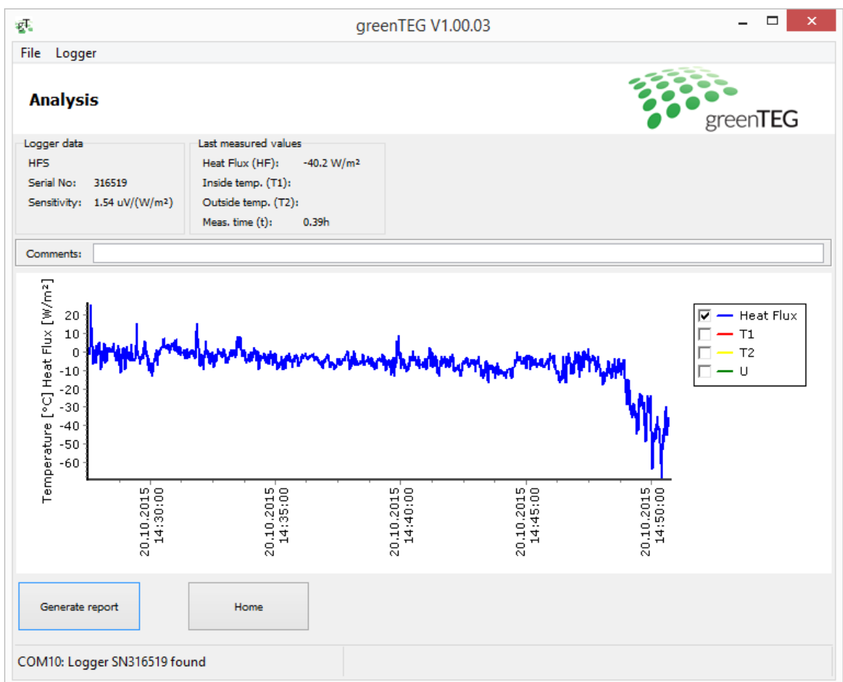
Figure 4: Analysis window showing heat flux output
